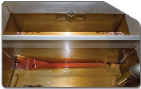
Hydraulic reservoir after moderate use with a conventional hydraulic fluid
