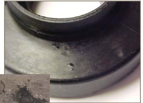
Pitting on filter end-cap
