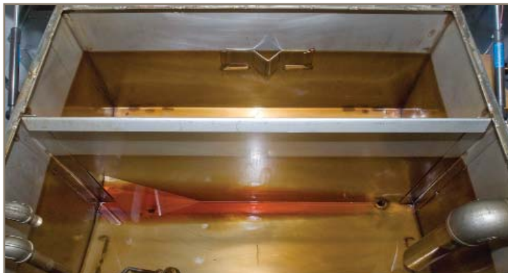
Varnish is attracted to metal surfaces, this results in an overall decrease in productivity.
