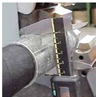
Measurement 1 in the plane of force
