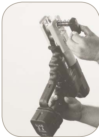
Open the retaining pin at the front of the machine by pressing the jaw release button
