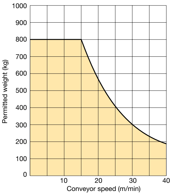
Loads - Moving mass subject to speed – Type STVSR-80-40
