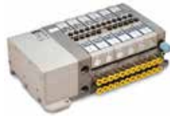
Up to 32 solenoid valves per island
